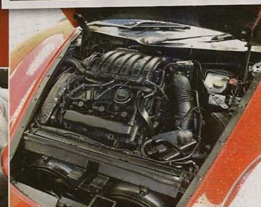
Paul Belk's V6 Peugeot lump boasts 210bhp and front wheel drive. Looks like quite a squeeze up front, but the bonnet does close and panel fit is surprisingly good
