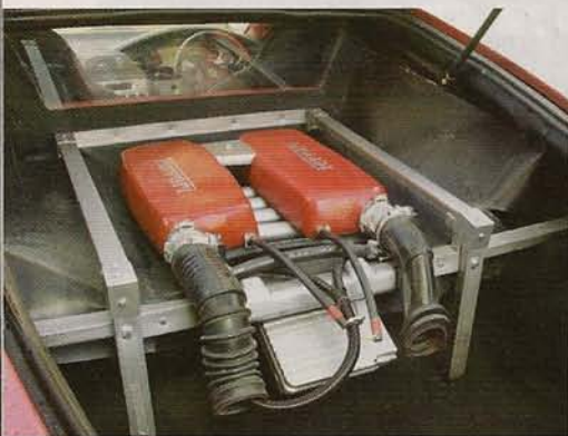
Fake Ferrari air boxes sit where the rear seats were fitted on the 406 – you can see them via cutout above
